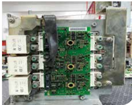
Replaced IGBT block
