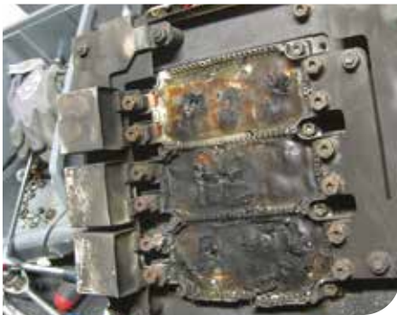
Damaged IGBT block
