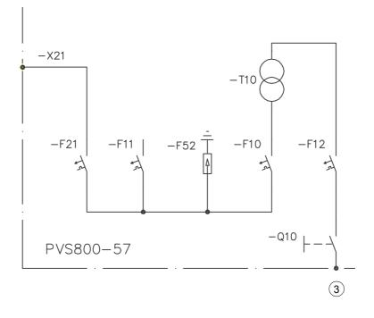
Auxiliary power supply from the inverter main circuit (option +G415)
