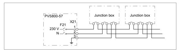
The maximum allowed current that can be connected to the power supply is 6 A.
