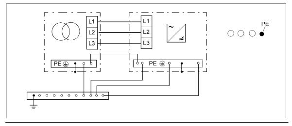
WARNING! Ground all conductive cable supports, cable clamps and individual conductive items close to cables, such as cable trays. A dangerous voltage can become present on the non-conductive outer sheath of the cable. This can cause injury or death.
