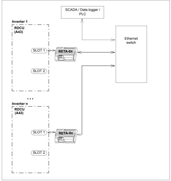
The diagram below shows a connection example for SCADA, PLC or data logger when a Modbus/TCP connection is used.
