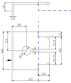
Clamp dimensions in millimetres. The dotted line denotes the cabinet frame.
